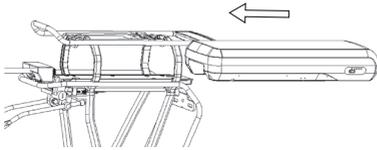
3. Once the battery is inserted, the battery can be locked. Then remove the key to avoid losing or damaging
